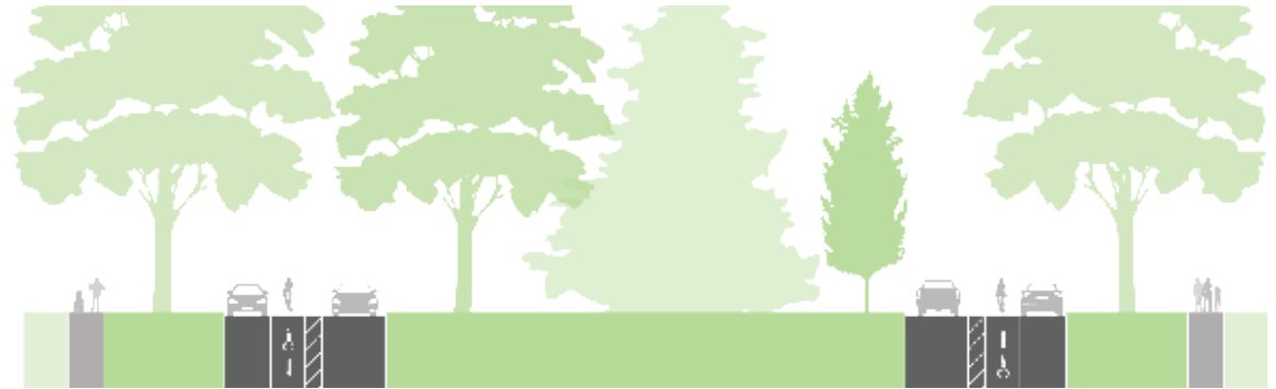
Fig. 3-27 | Typical 200-foot ROW with single median
