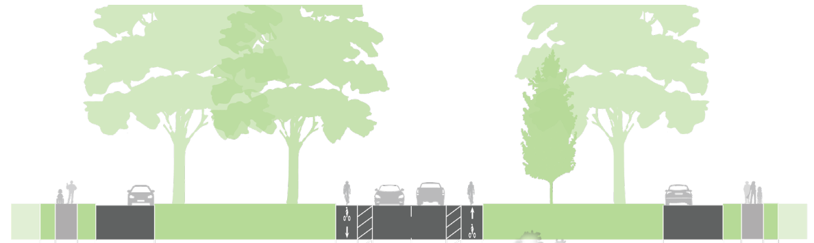
Fig. 3-28 | Typical 200-foot ROW with double median
